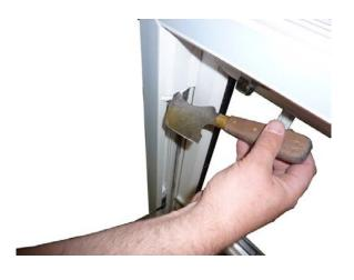
Carefully remove the end cover cap from the frame stop taking care not to damage the frame or sash stop
